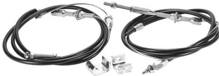
Figure 13 – Universal Emergency Brake Cable Kit (p/n: HWC2500)
