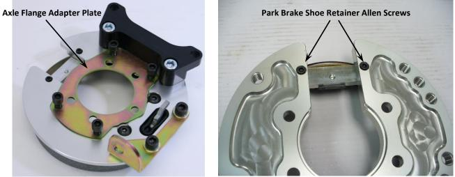
Figure 1 – Banksia Park Brake Assembly Reference
