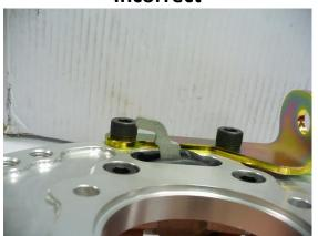
Figure 2b – Incorrect Cable Lever
