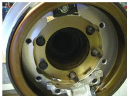
Figure 3 – Adapter Plate and Park Brake Assembly Installed on Axle Housing
