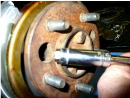
Figure 4 – Using the Access Hole
