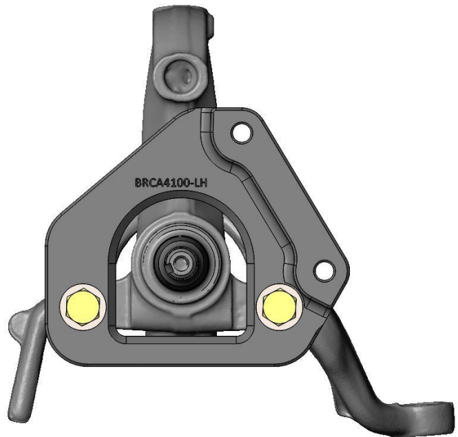
Figure 1b – Secondary Caliper Mounting Bracket Assembly Installed On Spindle (LH Shown)
