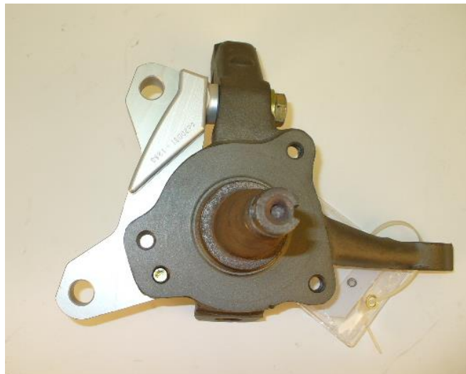
Figure 1 – Bracket Installed on the Spindle
