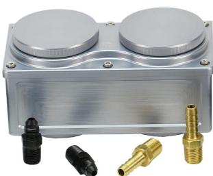
Thank you for purchasing the Master Power Brakes Billet Aluminum Reservoir Kit. This is a great and stylish way to provide a remote mounted fluid reservoir for your brake system when the master cylinder is mounted in a position that is not accessible. The reservoir is CNC machined from 6061 aluminum with a dual chamber design featuring individual o-ring sealed lids.
