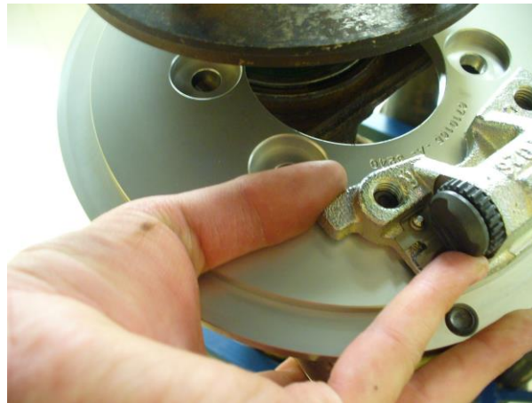
Figure 2 – Installing the Park Brake Backing Plate
