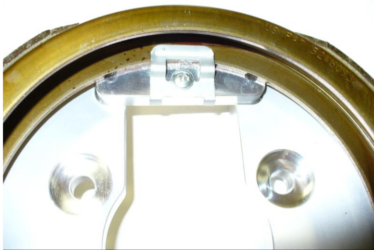
Figure 4 – Installed Park Brake Shoe Upper Retainer
