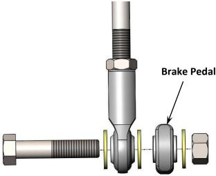
Figure 5 - Push Rod Attachment
