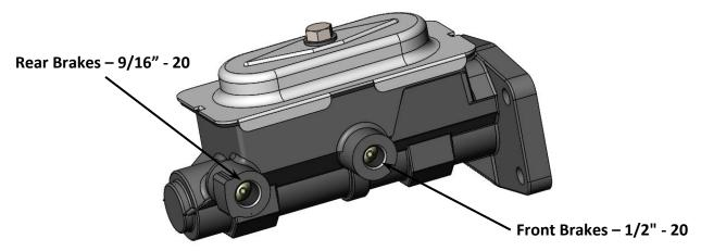
Figure 2 - Master Cylinder Port Diagram
