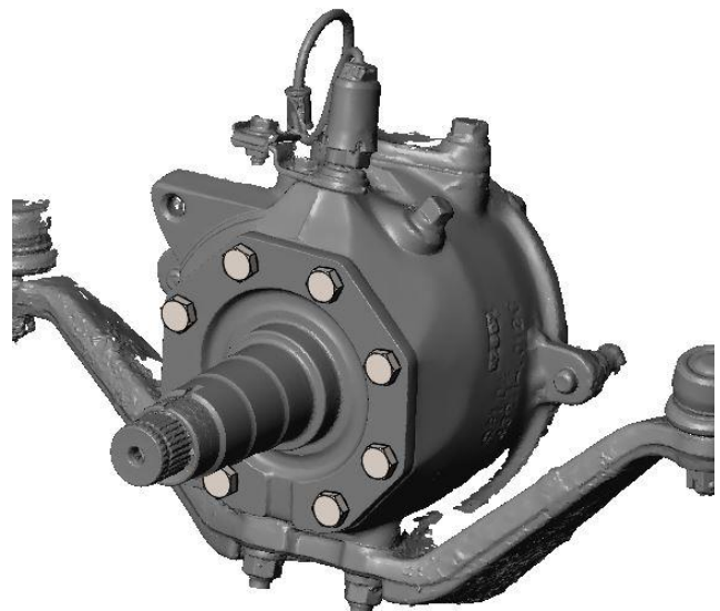
Figure 1b – OEM Stamped Steel Backing Plate Removed
